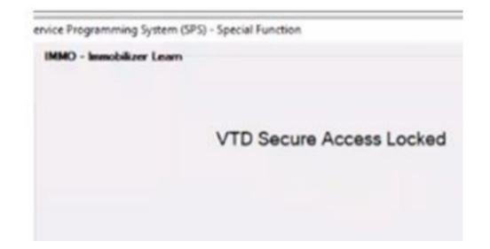
3. If a vehicle will not complete the SDAC, run the SDAC (using the Serial Data Authentication selection in Techline Connect) again. Select the box in SPS controller list in the lower right-hand corner labeled "Serial Data Authentication Configuration".
