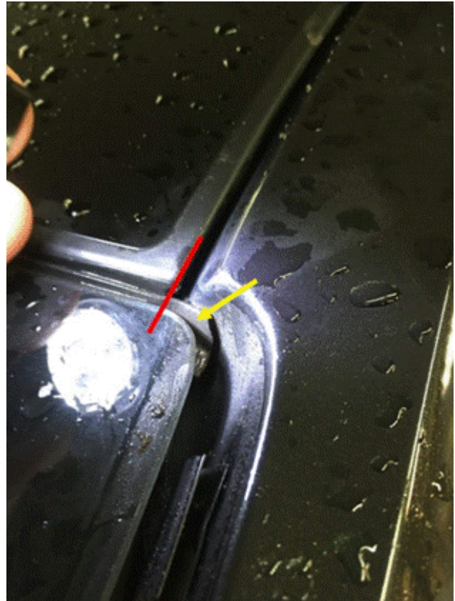
Figure 13. Section of windshield profile lip seal section to be cut away and removed.
