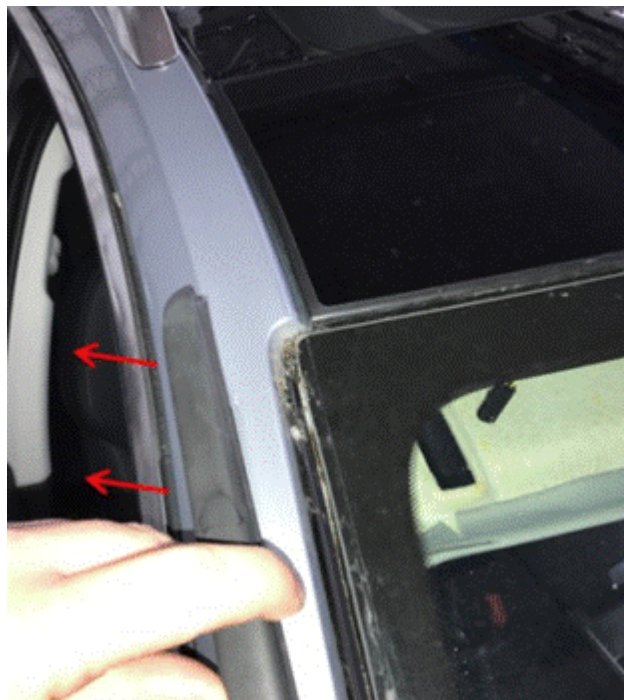
Figure 6. Drip rail removed.
