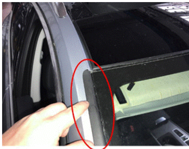
Figure 5. Drip rails to be removed.
