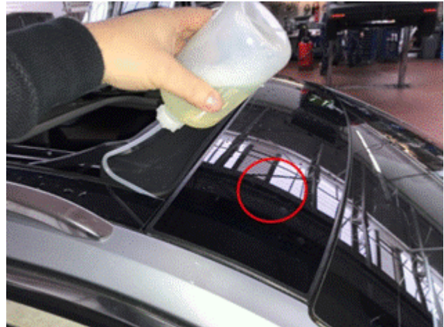
Figure 11. Mild detergent and water solution application.
