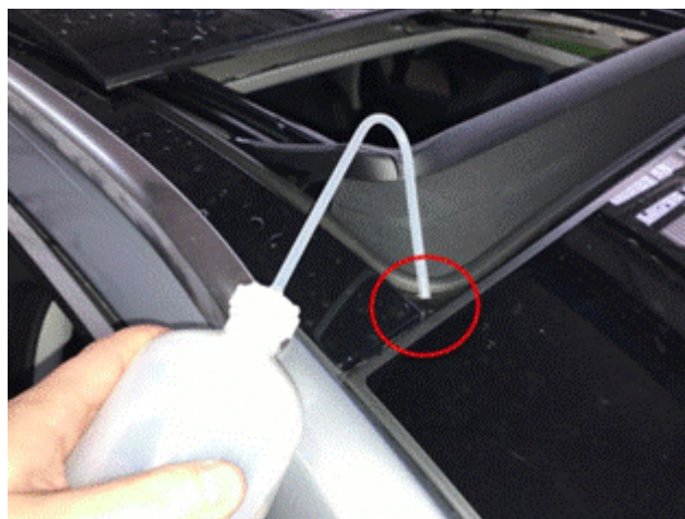
Figure 10. Rinsing the drainage channels.
