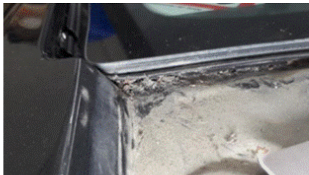
Figure 4. Drainage path obstructed.
