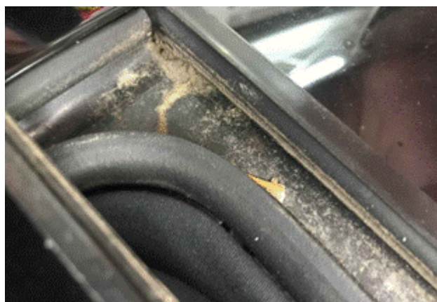
Figure 2. Sunroof frame drainage with the presence of fine dirt and debris.
