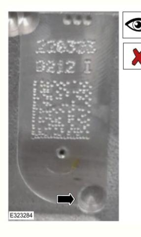
6. The failure condition shown highlights 3 drilled tooling marks in the upper, middle and lower right side of the tooling stamp.
