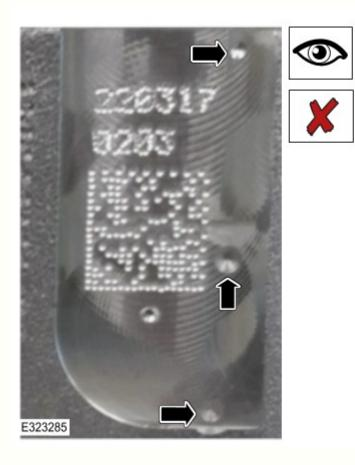
7. The failure condition shown highlights 2 drilled tooling marks in the upper and middle right side of the tooling stamp.
