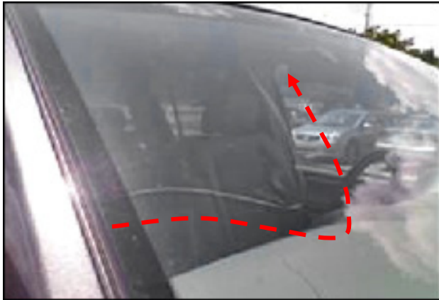
Single crack with no impact mark: Warranty
