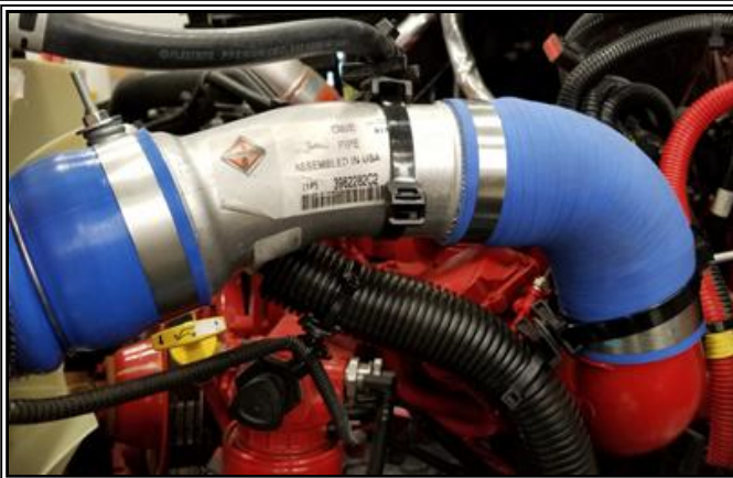
Figure 1: New CAC piping installed
