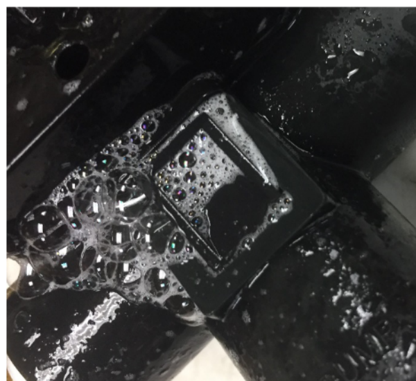
Examples of Acceptable Leakage at dump port flapper Amount of bubbles applies to all locations
