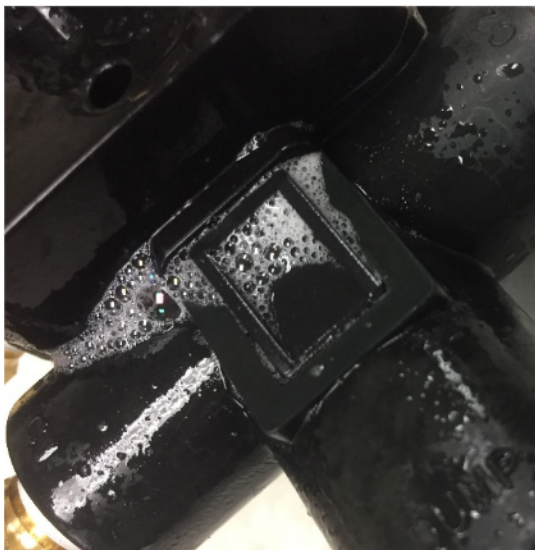
Examples of Acceptable Leakage at dump port flapper Amount of bubbles applies to all locations
