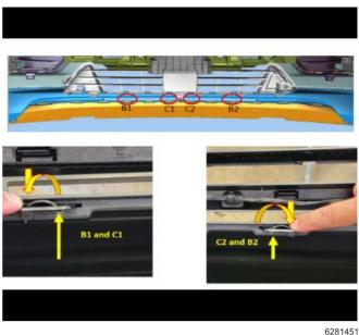
For locations B1-B2 and C1-C2 the zip tie knot needs to be facing down so as not to be visible to customer through grille opening above the skid plate.
