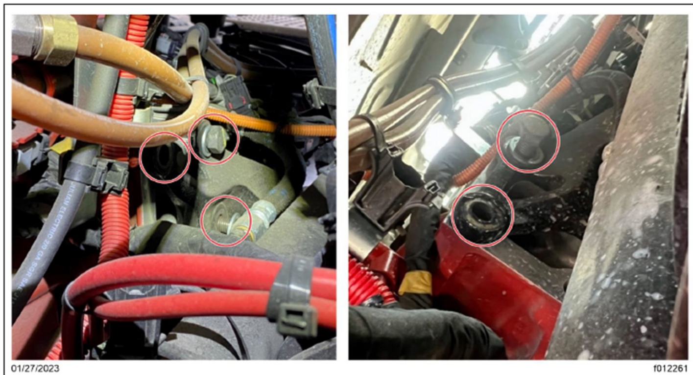
Fig. 1, Loose or Missing Rear Engine Mounting Bolts
