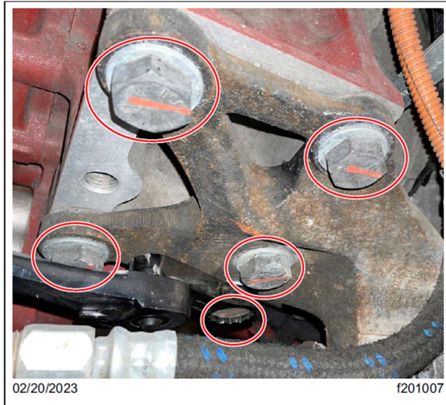
Fig. 3, Five Bolts with Torque Tool Attached
