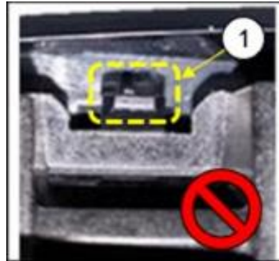
DETAIL A (1) Damaged tab
