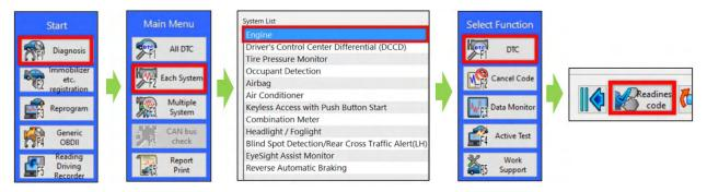
**P.** Read the readiness codes for P0016, P0017, P0018, P0019, P000A, P000B, P000C, and P000D. Confirm the self-diagnosis is complete and that the codes are not pending.
