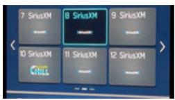
On all vehicles equipped with a CP 1.5 head unit ('23 Legacy/ Outback/Ascent) the SXM channels presets will not show the specific SXM channel logos when the vehicle is new. **This is a normal condition**.
