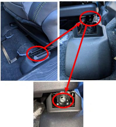
If the motor to raise and lower the seat bottom fails, there is no manual 'adjustment screw' available. The technician will need to remove the seat side cover and physically unbolt/remove the motor.
