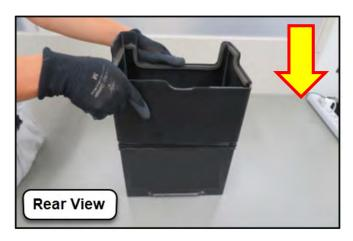
STEP 5: Assemble the ORIGINAL battery holder, NEW rear holding rod (p.n. 82161SJ000), and the ORIGINAL front holding rod as shown below. The original rod nut can be transferred to the new rear holding rod.
