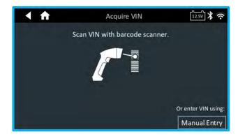
**NOTE:** In a case where the scanner option is unavailable the VIN can be entered by using the manual entry function.
