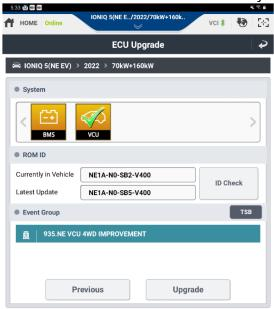
b. After the ECU Upgrade process shows 100% complete, cycle the ignition key to **OFF** for at least 10 seconds to reset the control unit.
