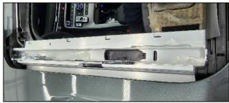
14. Install the new curve guide A (J) into the sunroof mechanism rail.
