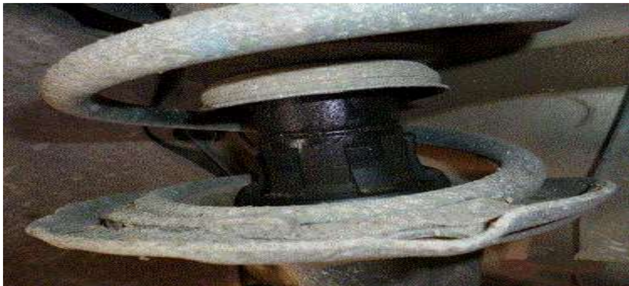
Figure 3) Not a leaking shock/strut
