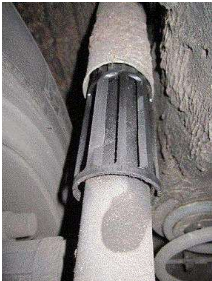
Figure 4) Not a leaking shock/strut
