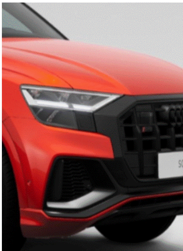
Figure 1. L1RR Platinum Grey radiator grille trim installed. LY9B Brilliant Black trim intended.
