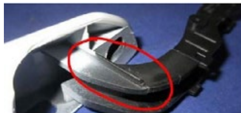
Figure 7. The door handle guide piece to be replaced.
