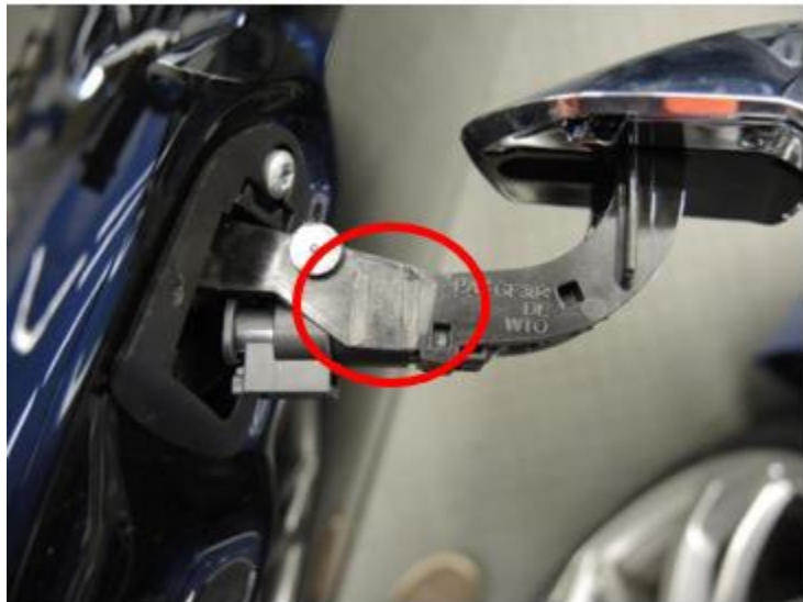
Figure 3. The door handle is shown with #1 and #2 ribs removed, leaving an even surface.
