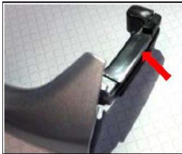
Figure 6. Top of rib #3 to be sanded down.
