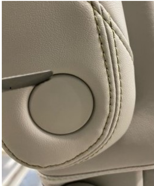
Fig. 1 Checking Gap With Go-No-Go Gauge
