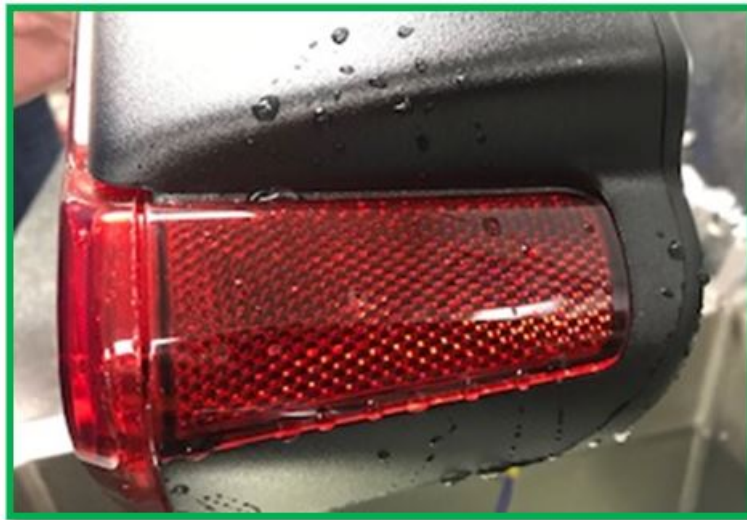
Fig. 3 No Water in Side Marker
