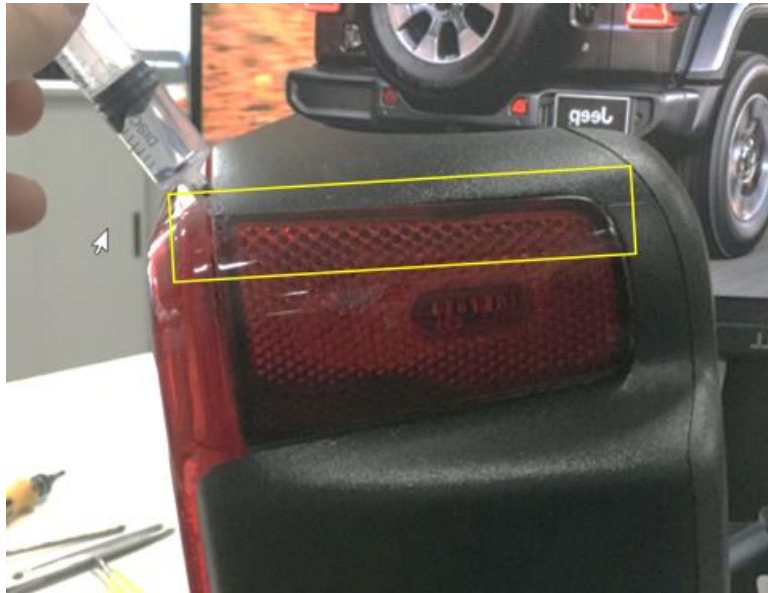
Fig. 1 Location of Water Intrusion Area
