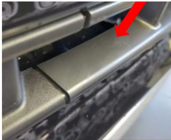
Fig. 3 Incorrect Center Grille With Smooth Surface
