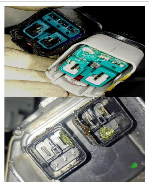
Examples of factory applied dielectric grease. Do not remove the grease.
