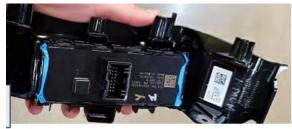
Driver side window switch and bezel (upside down view) with masking tape installed.
