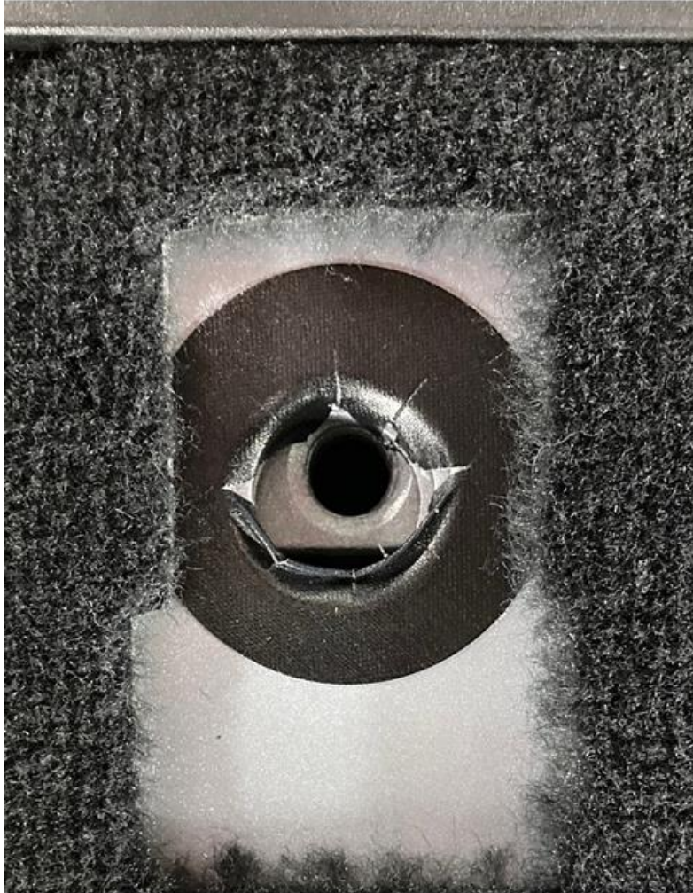
Fig 1 Seat Floating Cage Nut Do not remove the black tape patch material
