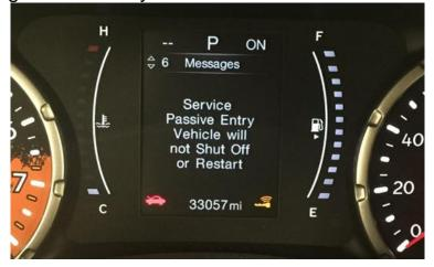
**Repair:** Engineering is currently working on a RFH software update with an anticipated release date in the <u>1st quarter of 2023</u>. **Replacement of the RFH or any other components will not resolve this issue.**
