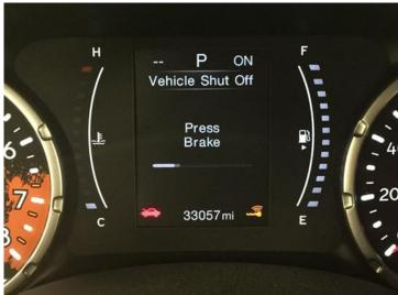
Step 5. First, press and hold the brake pedal AND THEN press and hold the OK button. The Press Brake timer will start.
