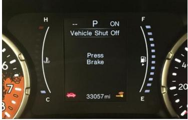
Step 4: Once the timer has completed and the "Press Brake" message is displayed. You must release the OK button.
