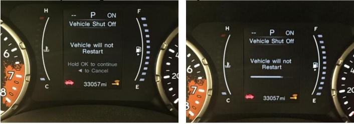
Step 3: The warning message that the vehicle will not restart is displayed. Press and HOLD the EVIC OK button. A timer bar will appear.
