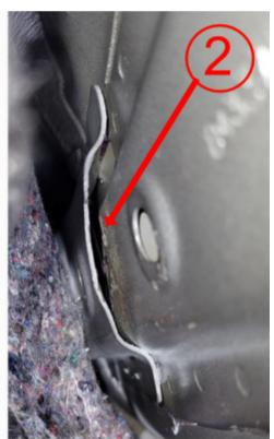
Apply a liberal amount of structural adhesive into the gap between the panels . Allow adhesive to cure overnight.
