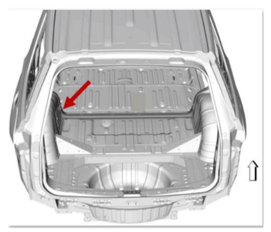
Inspect the area circled below for possible movement or itching of the body panels. You may be able to duplicate the noise by placing a crow bar in the gap between the panels and flexing the outer panel in and out slightly.
