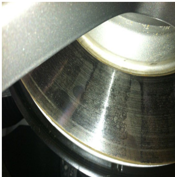
Figure 3. Discoloration on the brake disc due to chemical contamination from the cleaner that was sprayed directly onto the disc.
