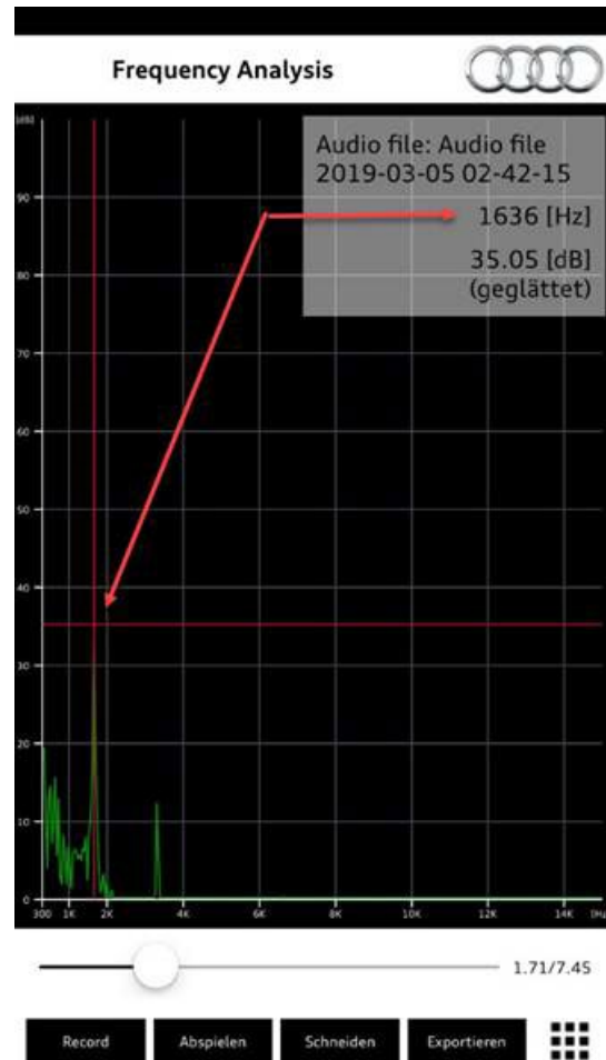
Figure 6. Example of a frequency analysis screenshot.
