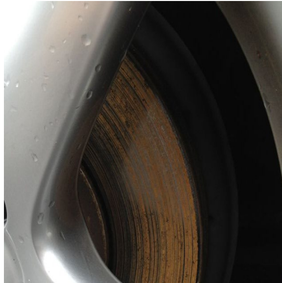
Figure 1. Disc covered with rust.
