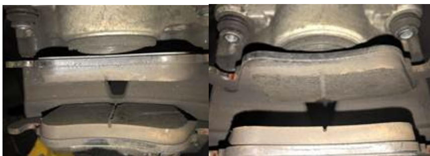
Figure 9 and 10. Example of Inner and outer with an adhesive pad.
