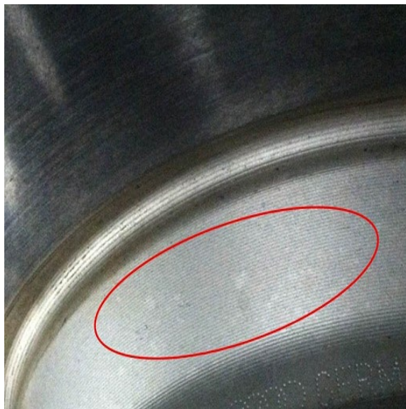
Figure 4. Small spots and discoloration due to chemical contamination from the cleaner that was sprayed directly onto the disc.
