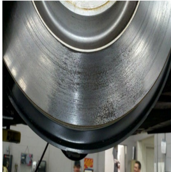
Figure 5. Brake pad material has transferred to the discs.
