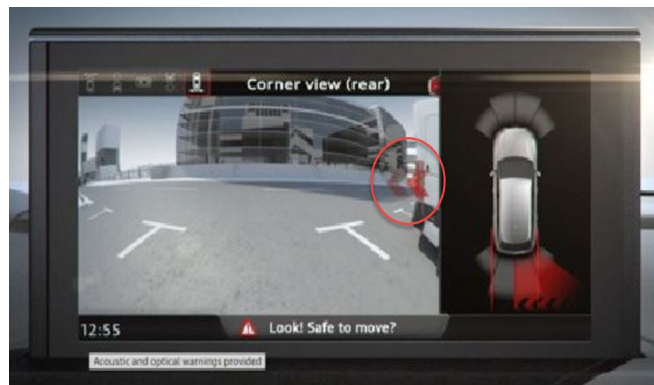
Figure 1: RCTA/Intersection assist arrows.
