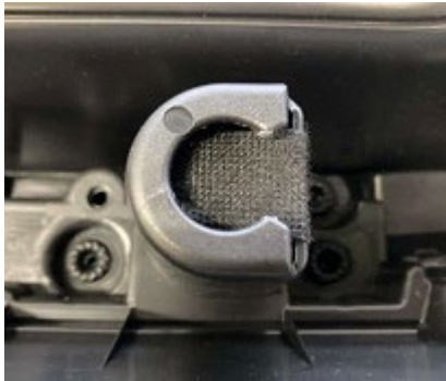
Figure 6. Door clip with fleece tape applied.
