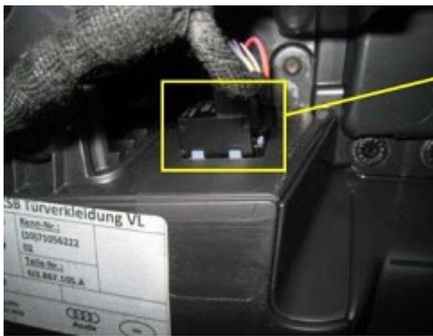
Figure 21. Apply fleece tape to pocket lighting.
