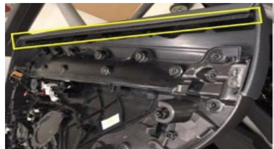
Figure 4. Fleece tape applied to mounting strip.
