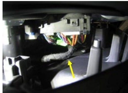
Figure 11. Wire harness contacting door trim panel.
