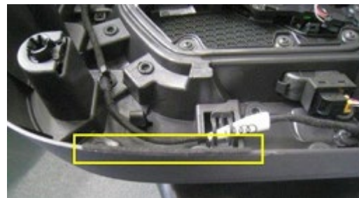
Figure 15. Felt tape installed on trim panel.
