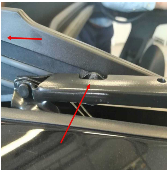
Figure 3. The left side of the slide and tilt mechanism.
