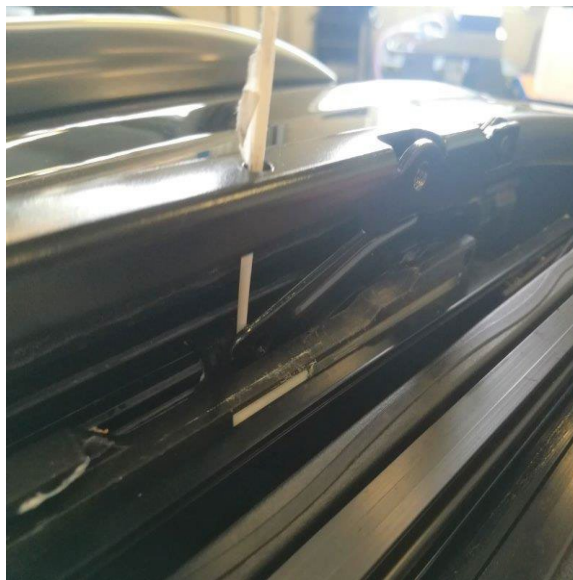
Figure 10. Close up view of the lubrication of the channel under the arm of the slide and tilt mechanism.
