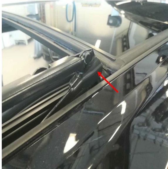
Figure 7. Section of slide and tilt mechanism to be lubricated.
