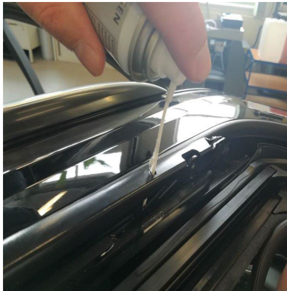
Figure 9. Accessing the channel through the arm of the slide and tilt mechanism.
