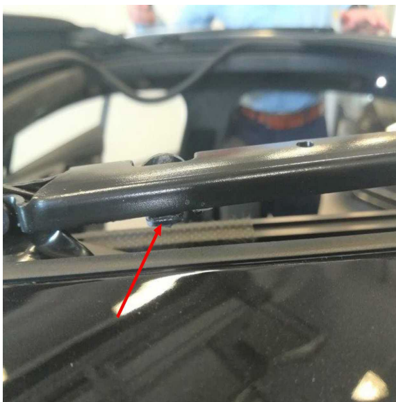
Figure 4. Lug to be lubricated on slide and tilt mechanism.
