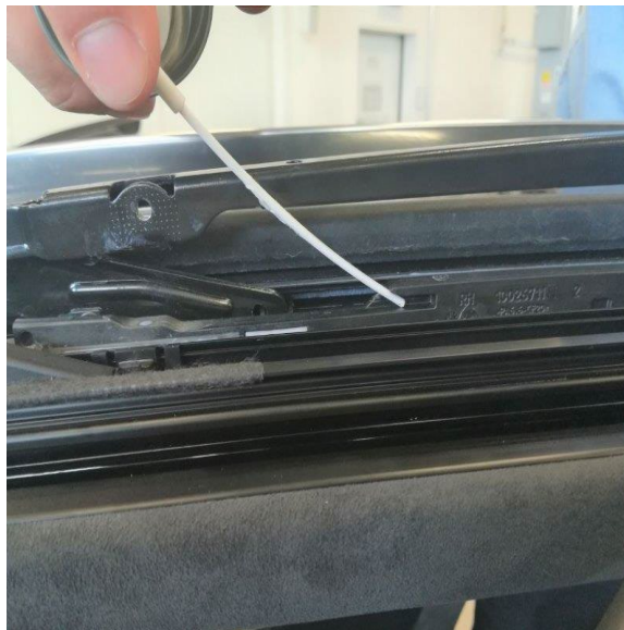
Figure 6. Lubricating the groove in the slide and tilt mechanism.
