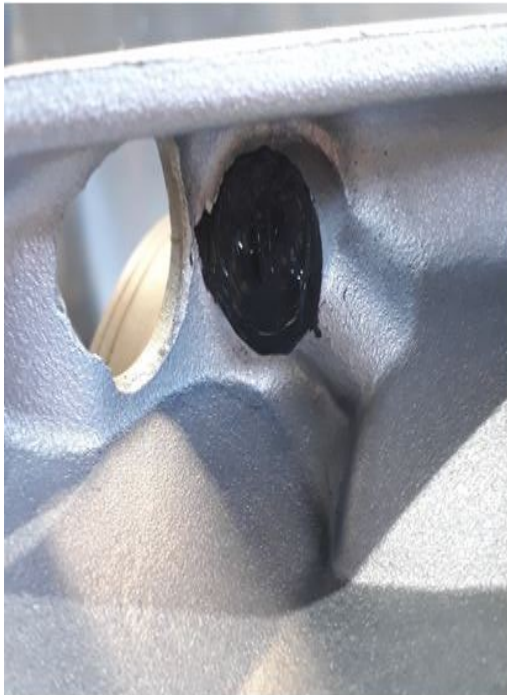
Figure 8. Silicone adhesive sealant example 1.
