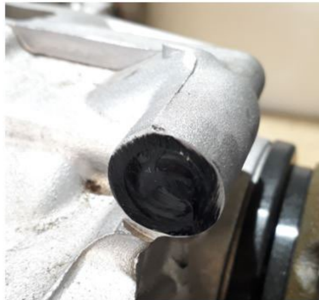
Figure 9. Silicone adhesive sealant example 2.
