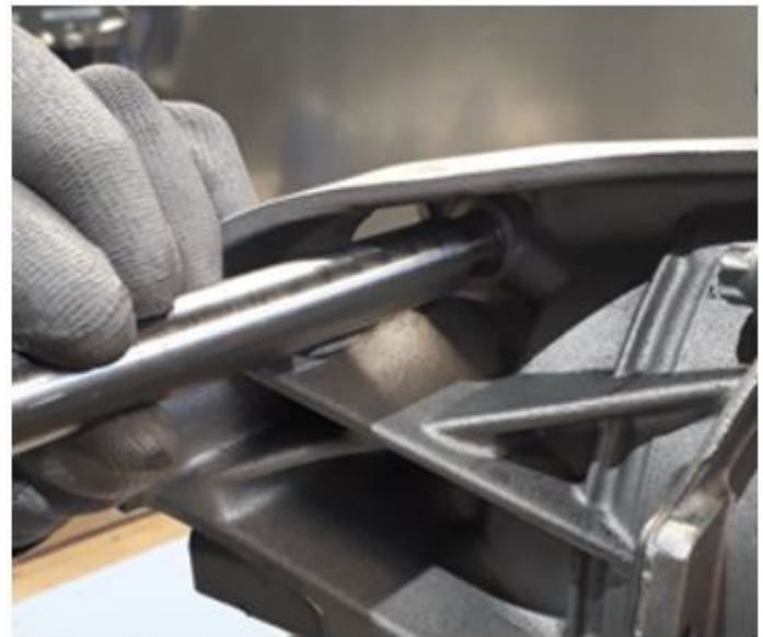
Figure 5. Installing sealing cap
