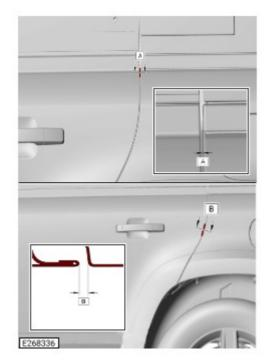
Check the alignment of the rear door(s) in the areas shown in the illustration.
