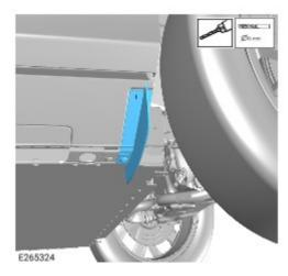
Using a 6 mm drill, create a hole through the left air deflector and the left rocker panel molding in the position marked during step 3.
