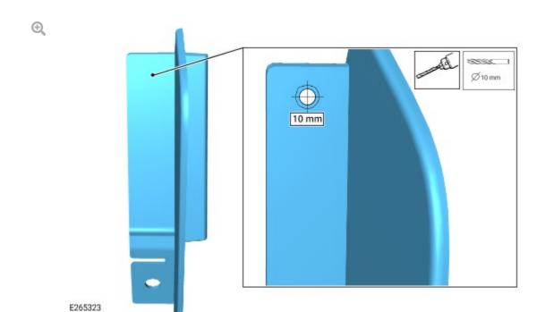
Using a 10 mm drill, increase the size of the new hole in the left air deflector from 6 mm to 10 mm.
