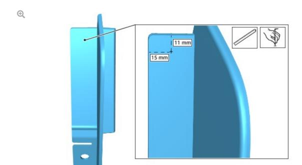
Measure and mark the position on the left air deflector for drilling, as shown in the illustration.
