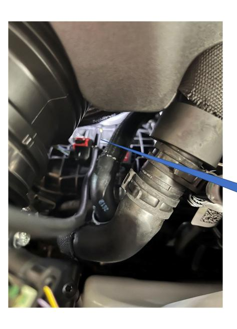
Using a suitable borescope, slide the end of the scope below the air intake on the left hand side, above the intake air sensor connector, just in front of the coolant hose.
