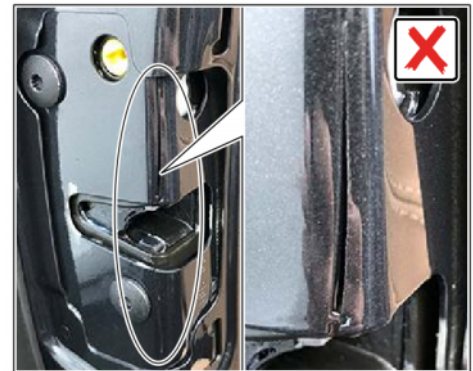
Checking lock reinforcement on rear left door
