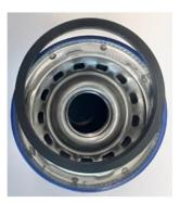
If any damage is found, replace the filter. If no damage is found, the seal may be refitted to the filter and installed on the vehicle.
