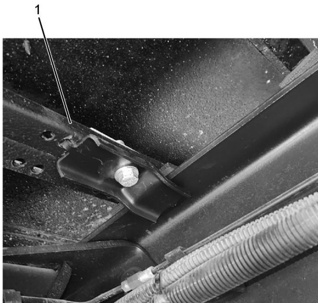
Figure 2. Body Tie-Down by the Rear Axle – Left-Hand Side
