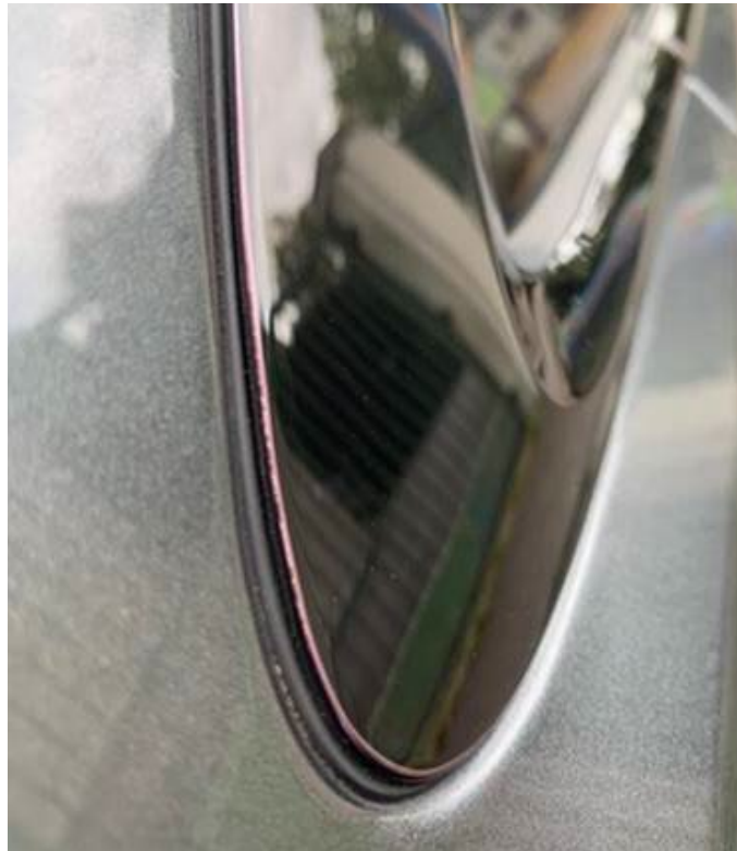
Figure 3. Discolored black optic trim around the rear side window.
