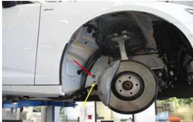
Figure 12. The yellow arrow indicates the opening where the borescope will be inserted to inspect the completeness of the sealant application.
