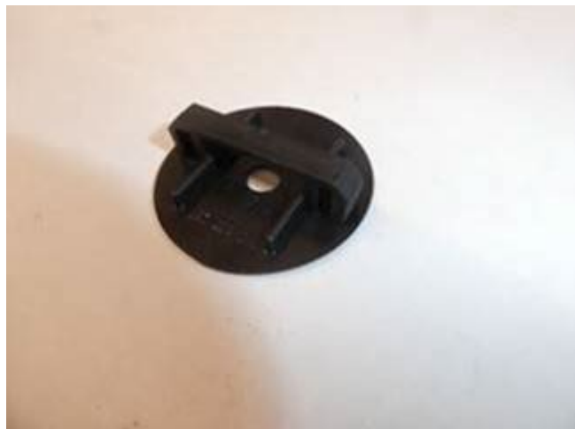
Figure 15. New longitudinal member plugs with integrated drain.
