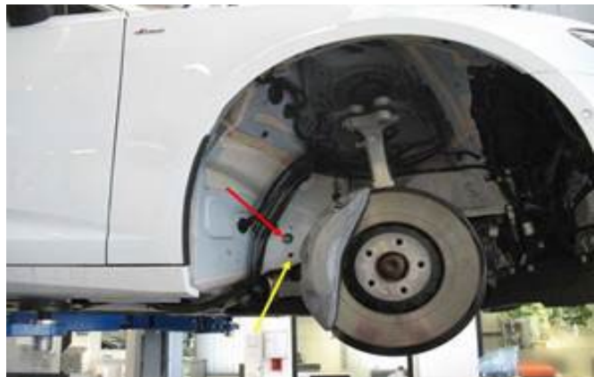
Figure 5. Point of entry for the borescope.
