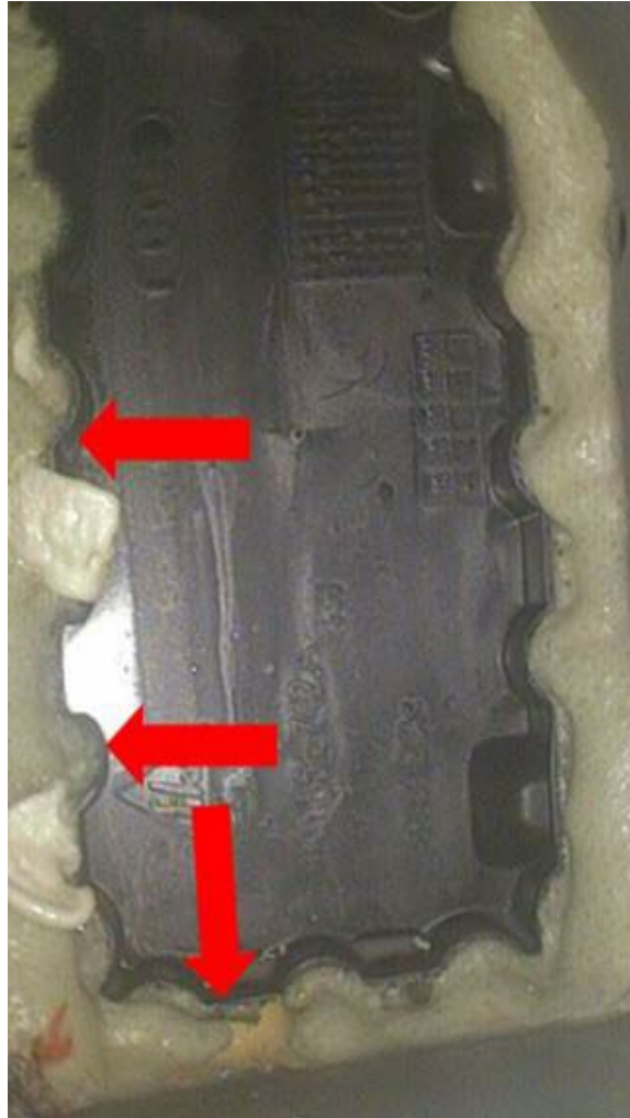
Figure 7. Sound absorber to be completely sealed off.
