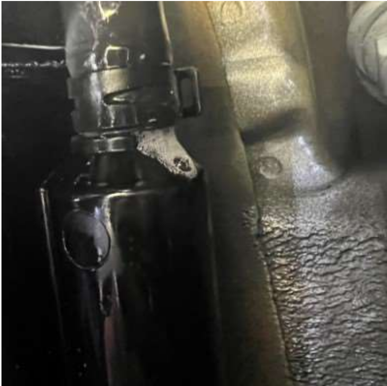
Figure 3. EVAP leak under a clip securing a connecting hose.
