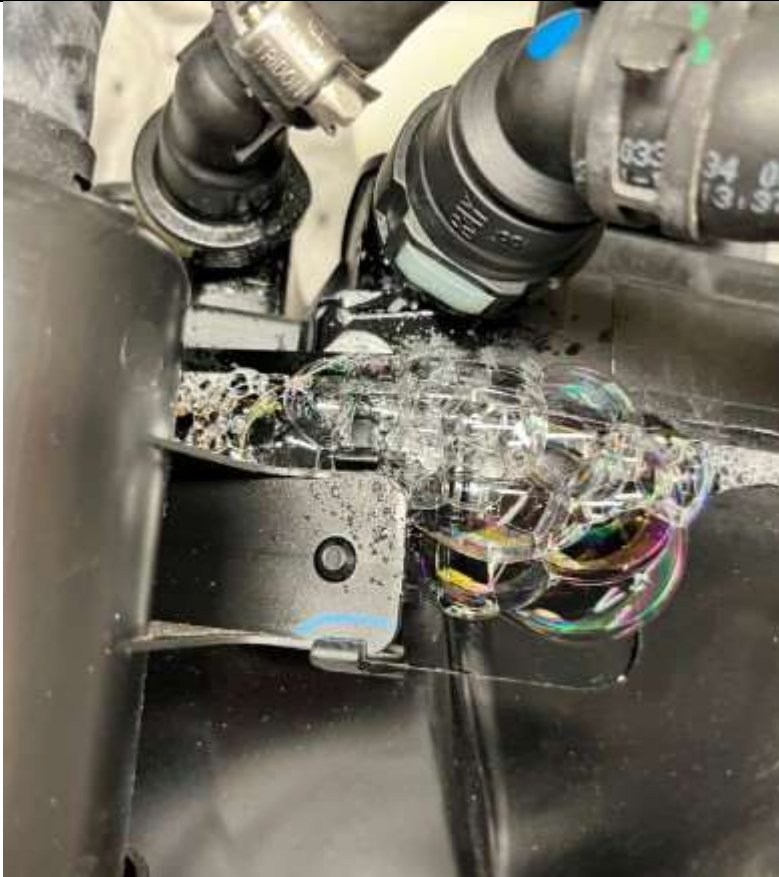
Figure 1. EVAP leak along the upper seam, by the fresh air filter securing bracket.
