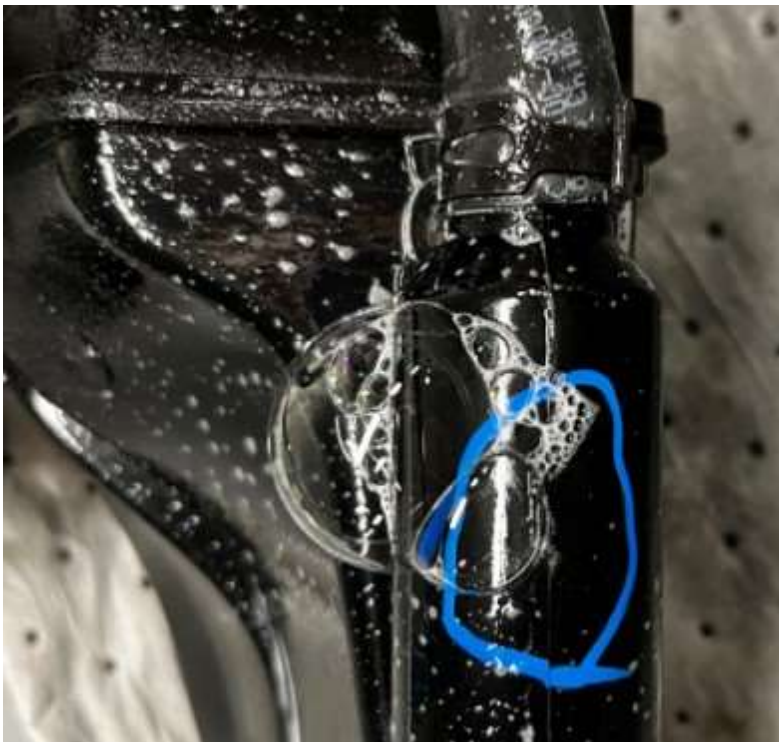
Figure 2. EVAP leak along the right-hand seam, near a connecting hose.
