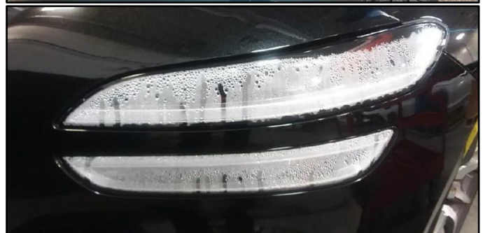
Water collecting inside the headlamp
