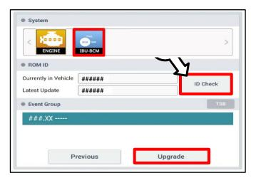
8. The ECU upgrade will begin and the progress of the upgrade will appear on the bar graph. Upgrade part (1/2) (E) will download the upgrade event to the VCI-II. Upgrade part (2/2) (F) will upgrade the ECU.
