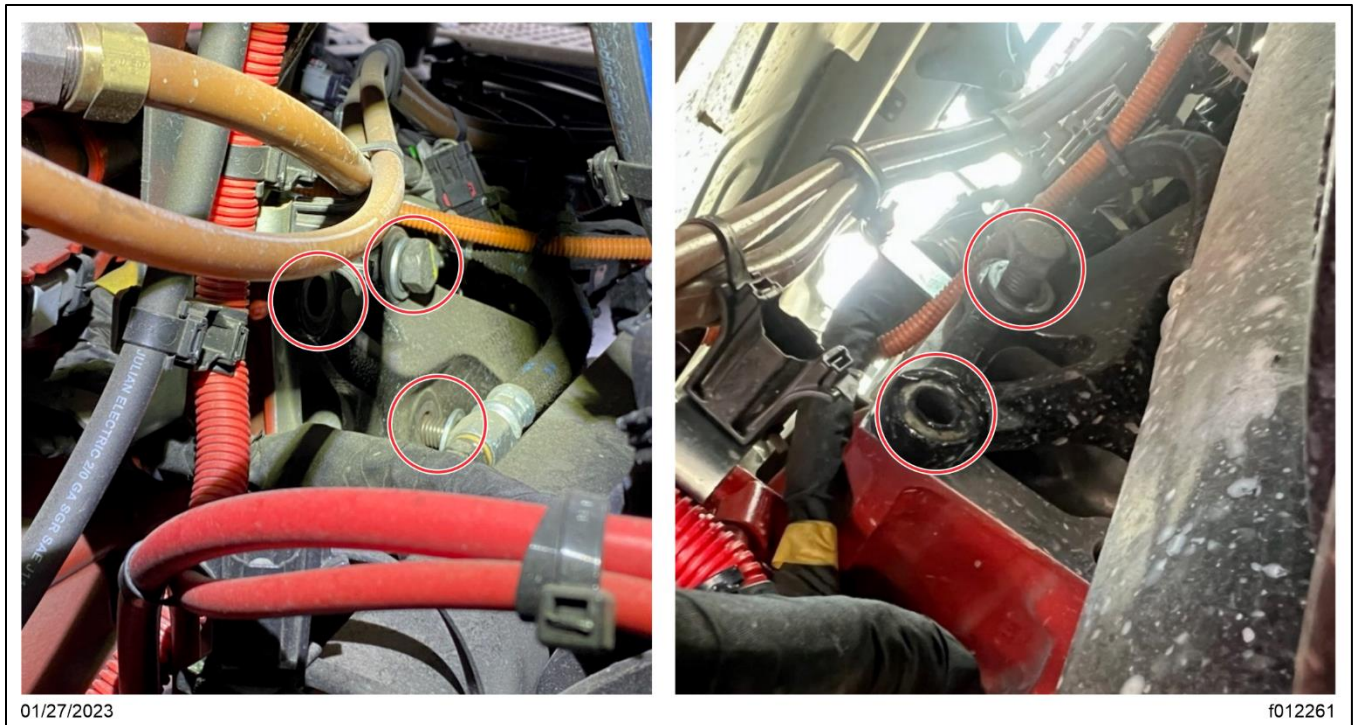
Fig. 1, Loose or Missing Rear Engine Mounting Bolts
