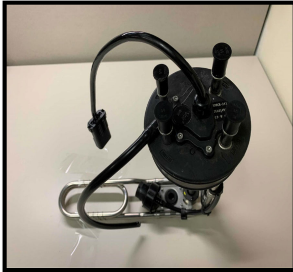
Figure 2, KUS Optical Header Quality Sensor with Cover
