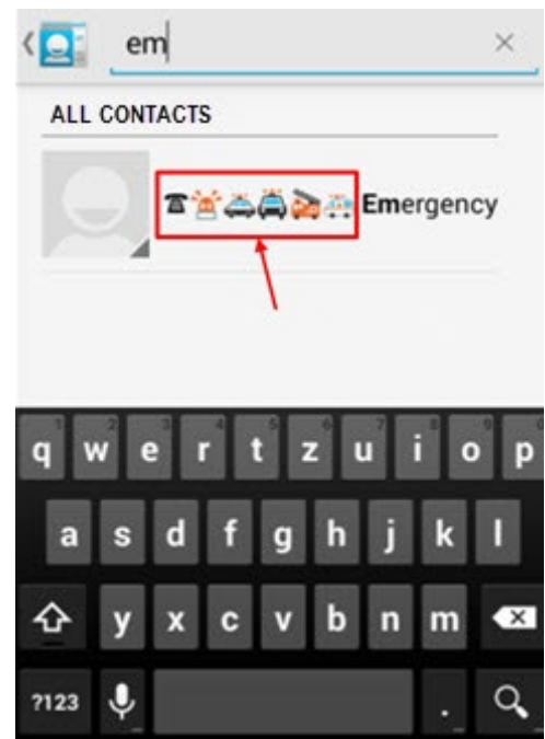
Figure 1. Special characters are stored in the name field of a phonebook contact.
