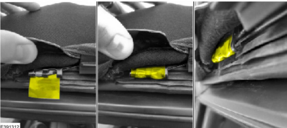
**11.** Install felt onto the rear quarter window.
