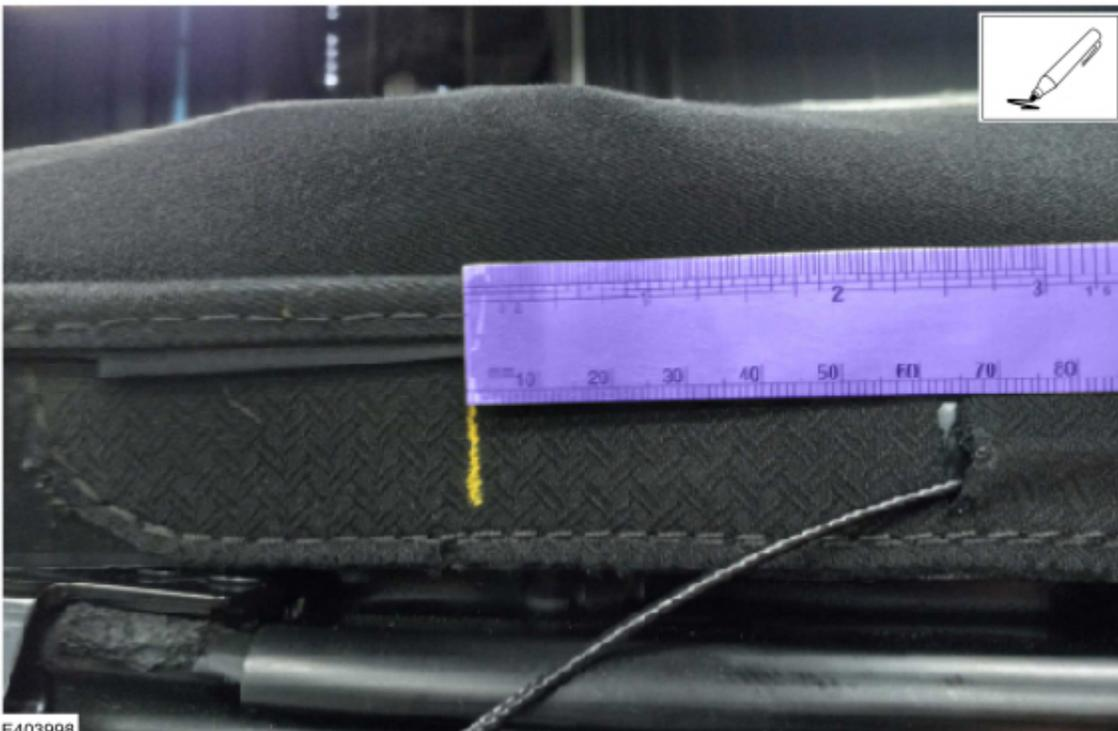
(2). Use a razor blade to cut a new vertical entry point at the location marked in the previous step. This entry point must be similar in size to the original entry point. Be sure not to damage the stitching (above and below the
