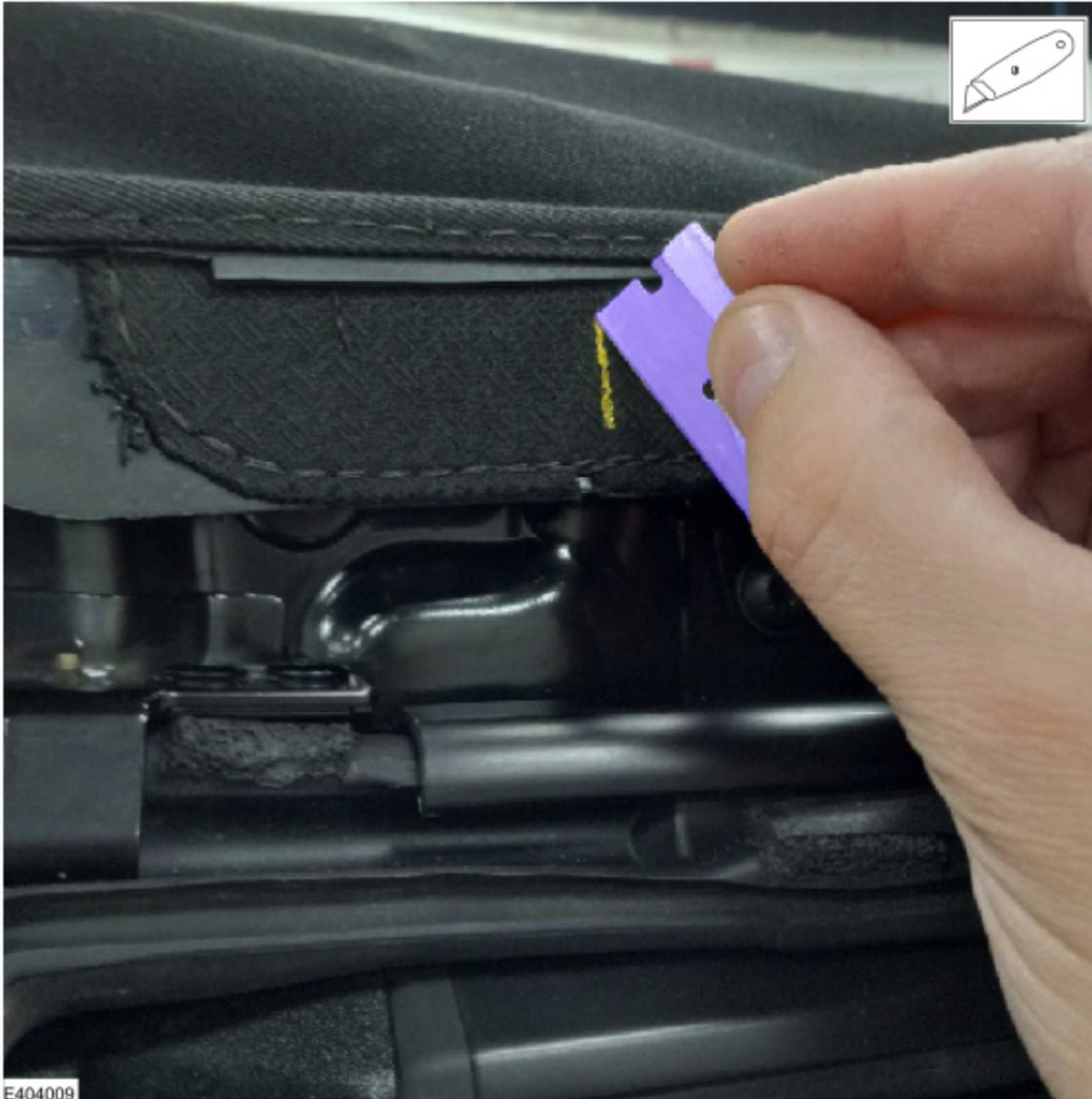
**8.** Install the new front and rear seal retainers (4 total). Refer to the Workshop Manual, Section 501-18A, Removal and Installation > Soft Top Seals and Retainers. During replacement, transfer the original seals onto the new seal retainers, apply Motorcraft® Threadlocker to all seal retainer fasteners. Completely remove and discard the original tension cable assembly from the soft top material.
