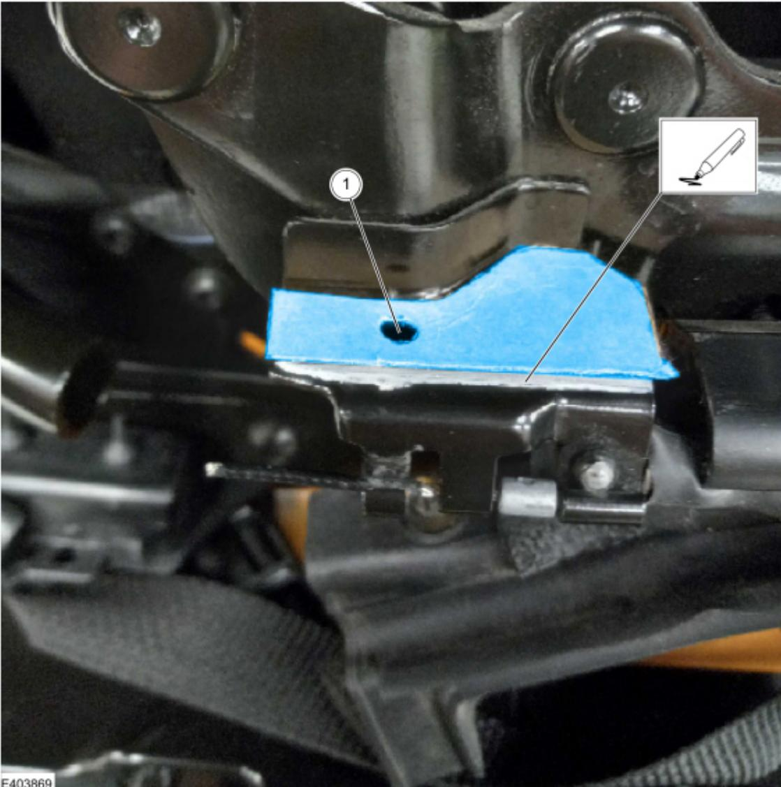
(5). Place protective material around the cable guide to prevent sparks and metal debris from contacting the vehicle. Be sure the soft top material is completely protected as any sparks that contact the material will cause damage.
