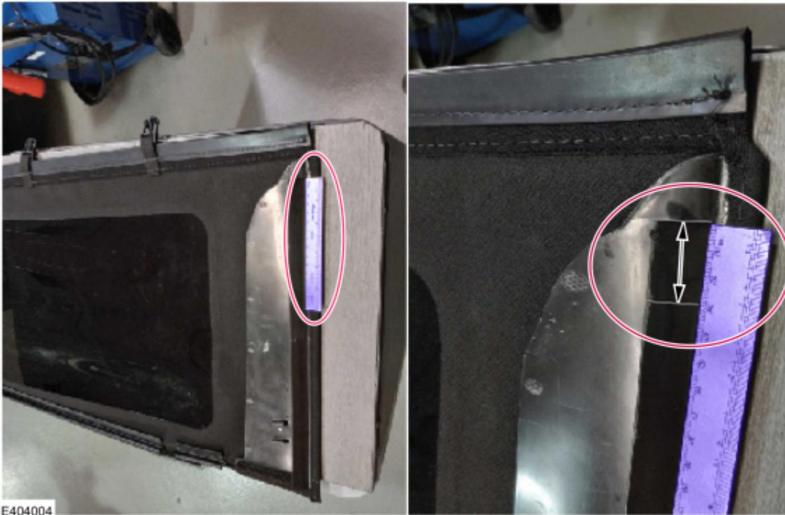
(5). Grab one felt strip (Figure 24, Callout 1) and peel the paper backing off, exposing the adhesive underneath. Install the felt on the previously marked line, keeping it centered in the channel. (Figure 30)
