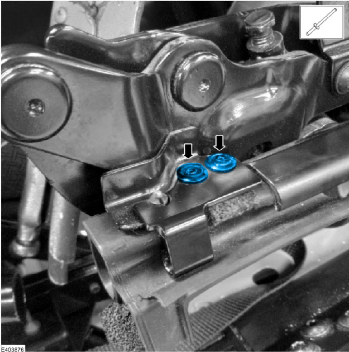
**5. Install the front tension cable rear linkage.**
