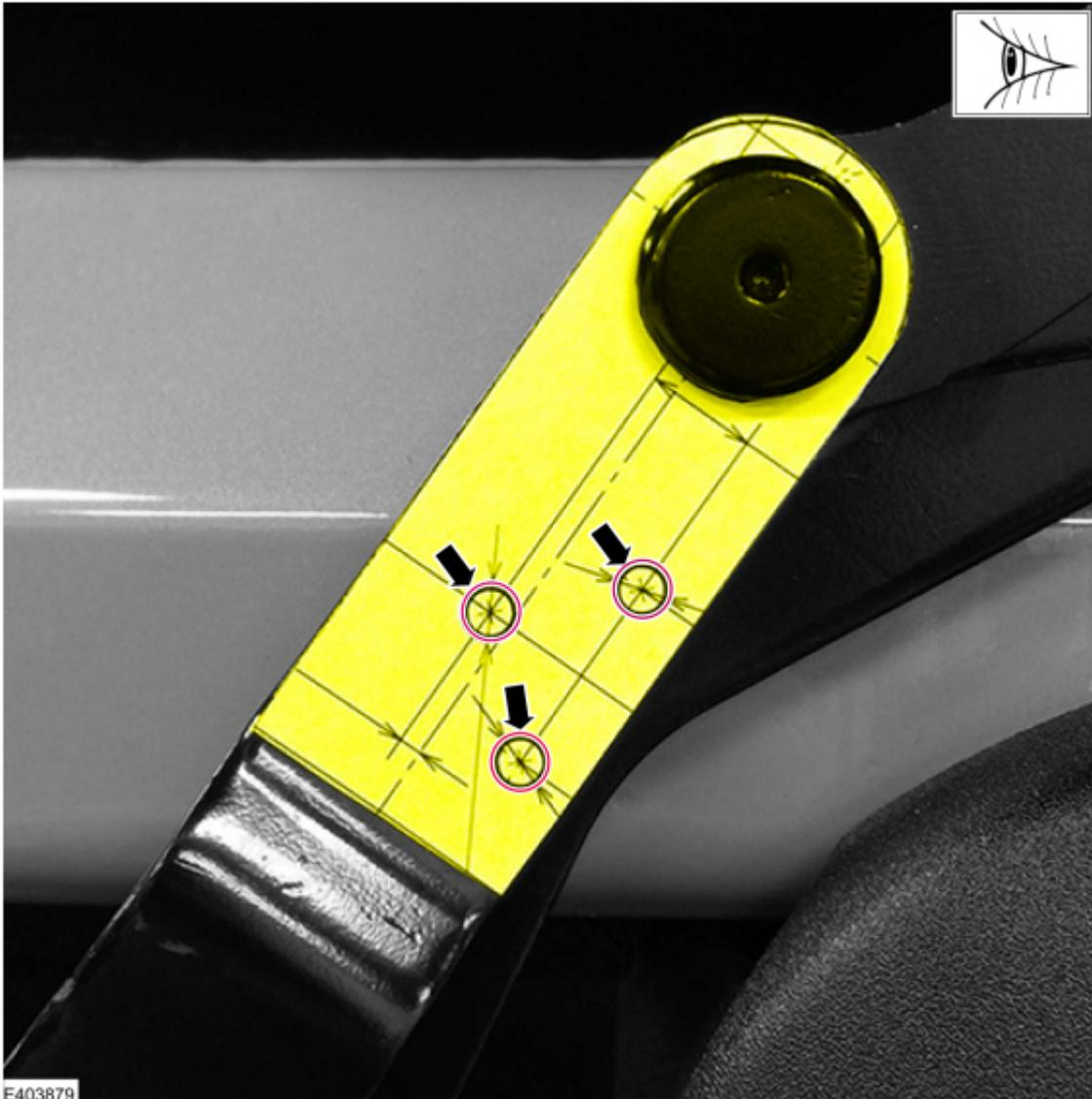
(5). Remove the template from the frame then use an 11/64 in. (4.2 mm) drill bit to drill holes in all 3 marked locations. While drilling, do not allow the drill bit to contact other frame linkages located directly behind this area.
