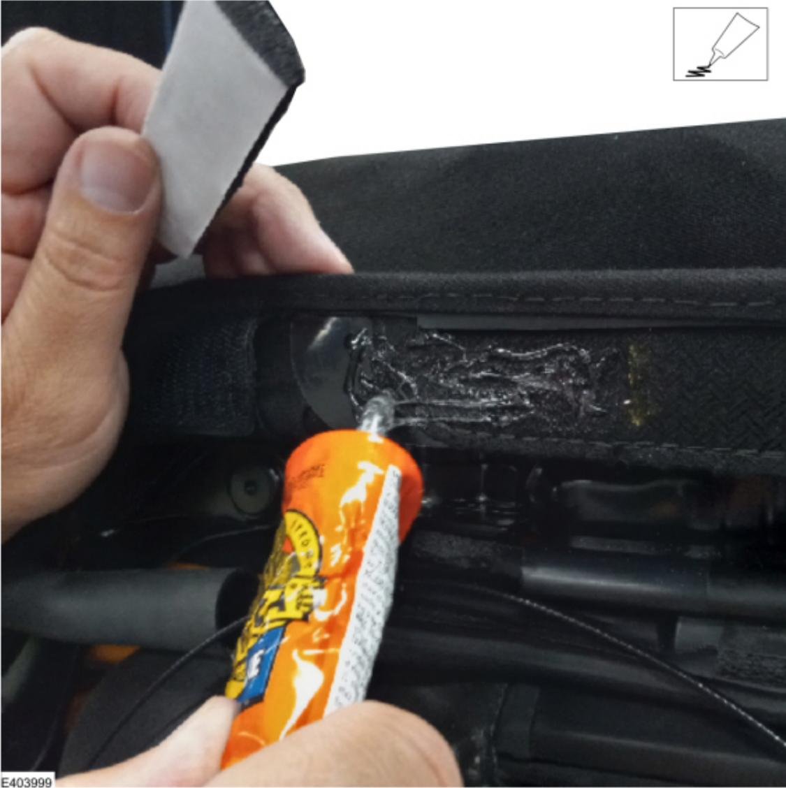
(3). Grab one foam strip (Figure 24, Callout 2) and peel the paper backing off, exposing the adhesive underneath. Install the foam onto the material. The foam must be installed just behind the new entry point created in Step 7. (Figures 24-25)
