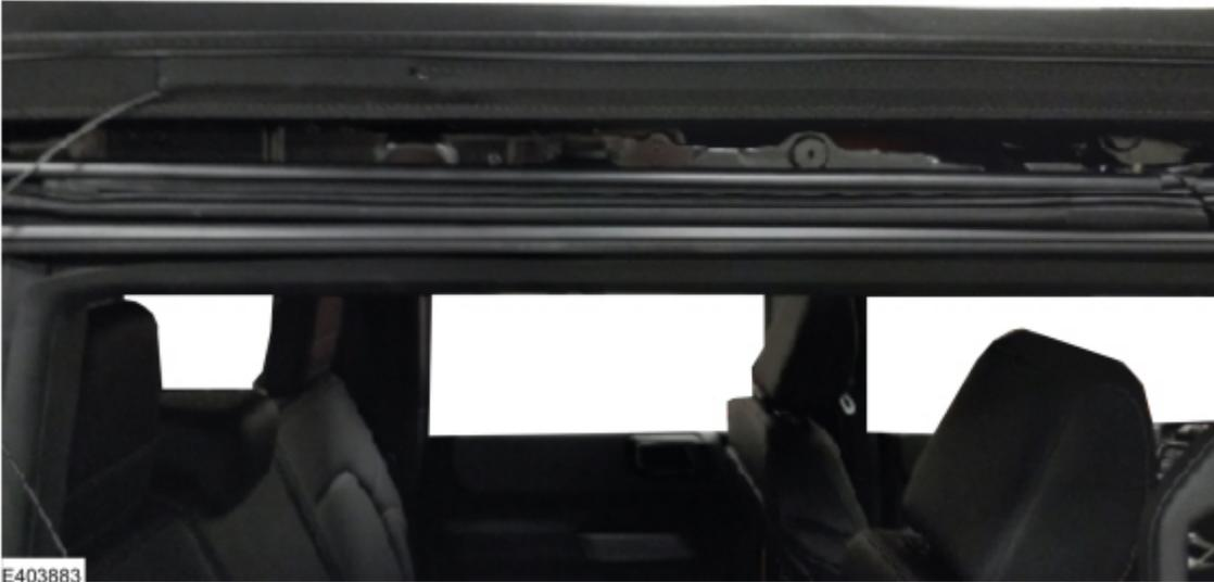
(3). With the entire length of the K-seal scored, pull the k-seal, separating it from the soft top material. The k-seal will tear along the previously scored line. If any large pieces of the seal remain, use the razor blade to carefully score those sections and remove them. (Figures 19-20)
