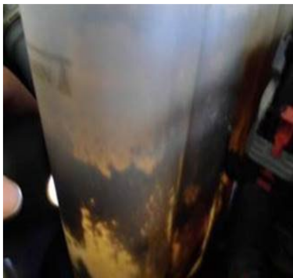
Figure 3. Discoloration on the inside of the coolant reservoir.
