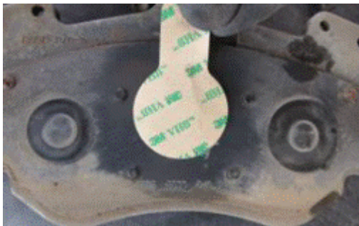
Figure 2: Adhesive location – center piston position in the brake pad.
