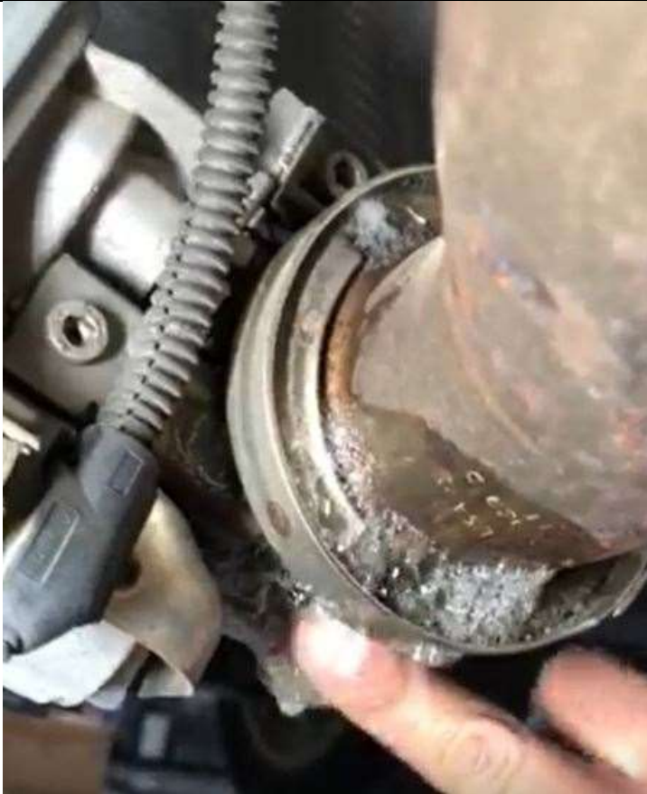
Figure 1. Example of exhaust leak at exhaust flap.
