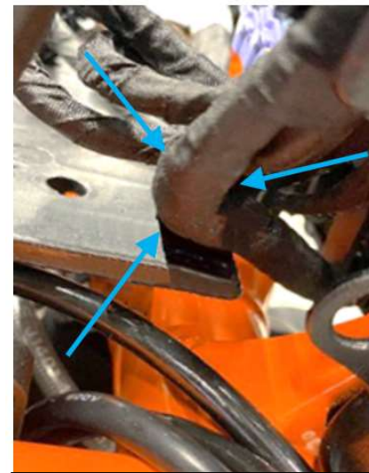
Area A1: Inspect the wiring for damage at the indicated location. Also check if the cable tie with foot section is missing or installed. (Take photo for claim)
